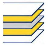
Release Liner Adhesive Carrier Adhesive Release Liner
